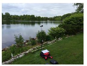
During the measurement, the SPL meter's microphone is facing toward the imaginary point of the sound source.
